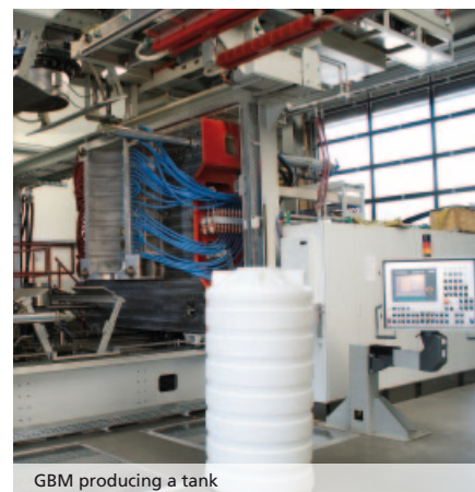
GBM producing a tank
